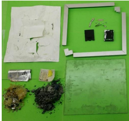
Figure 3: Macro components separated using organic solvent. Starting on the top left of the image and going clockwise: back sheet, frame, junction box (inside the frame), substrate, loose cell/encapsulant/filaments, scraped cell/encapsulant/filaments, property labels
